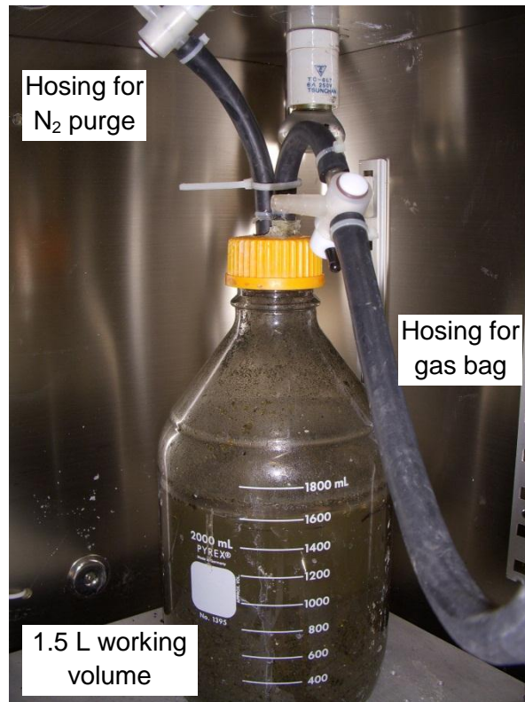
Figure A-1: Diagram of bench-scale anaerobic digesters
